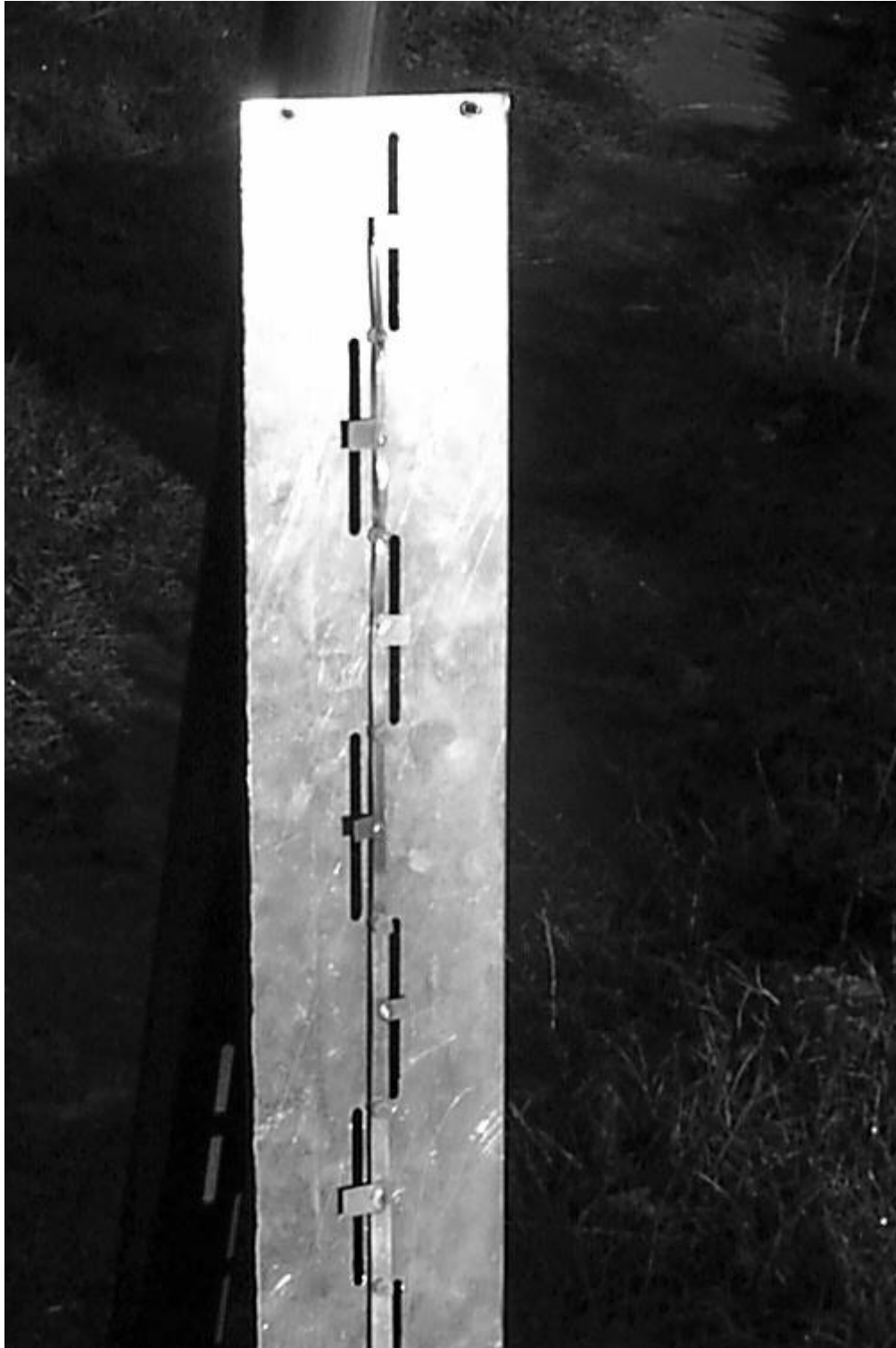
Fig 9 GB3MHS Slotted Transmission Line Antenna
