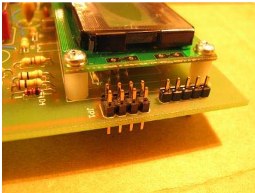
Fig 2 – View of partially constructed LC Meter, showing how JP1 and JP2 are installed, and mounting of LCD above PCB
